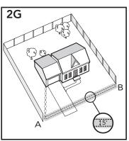
Sample 4 (2G): Front Boundary Only (Double Loop) From the Fence Transmitter, run the wire to A, A to B, B back to A keeping the wire separated at least 5 feet. Twist the wire from A back to the Fence Transmitter.
